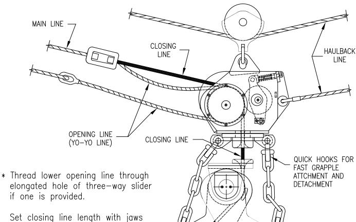
Set closing line length with jaws fully open, chains tight and threeway slider against carriage.
