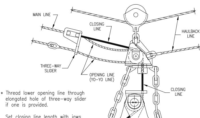
Set closing line length with jaws fully open, chains tight and three—way slider against carriage.
